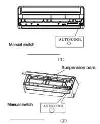
NOTE: The unit must be turned off before operating the manual control button. If the unit is operational, continue pressing the manual control button until the unit is off.
